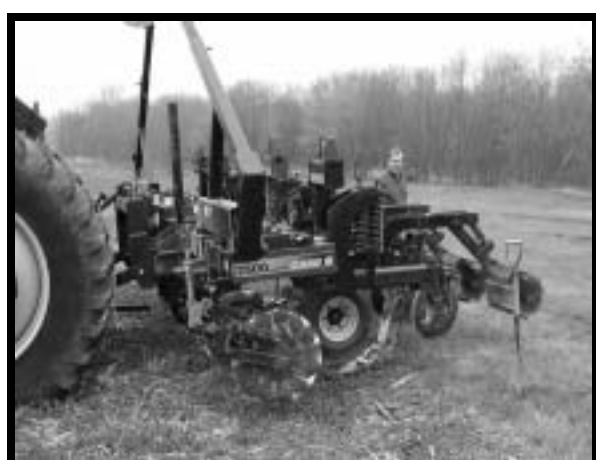
CASE-IH Ecolotill 2500 strip till unit with MRD shanks, hiller disks and rolling basket (used in 2002)
